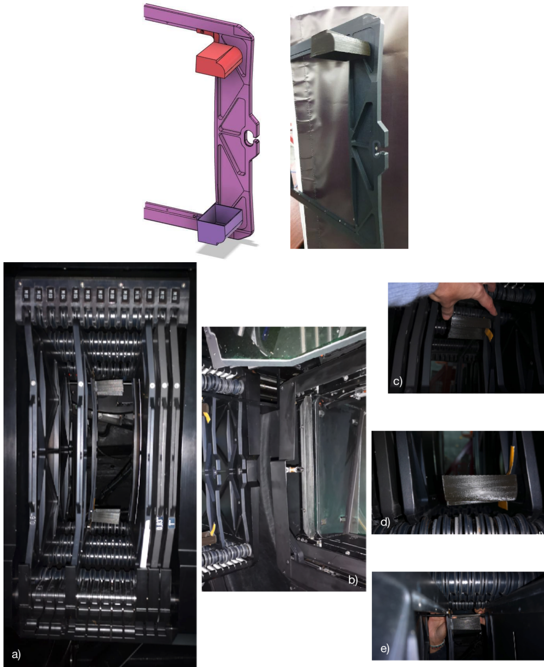
Figure 26. Top: 3D printed dummies built for the in situ testing of the MAAT envelope on OSIRIS (Credit: GTC). Bottom: In situ testing of the dummy of the MAAT module on OSIRIS: a) MAAT envelope dummy placed in the Loader mask, b) Baffle to redesign in order to accommodate the subsystem mask frame plus MAAT envelope, c) Width of the MAAT envelope, d) Free space between the rollers and the lower part of the MAAT envelope (orientation rotB = 80^\circ ), and e) Free space between the upper part of the MAAT envelope and the masks edge protection (orientation rotB = 80^\circ ). All these pictures have been taken with orientation of rotB = 80^\circ . (Credit: GTC).
