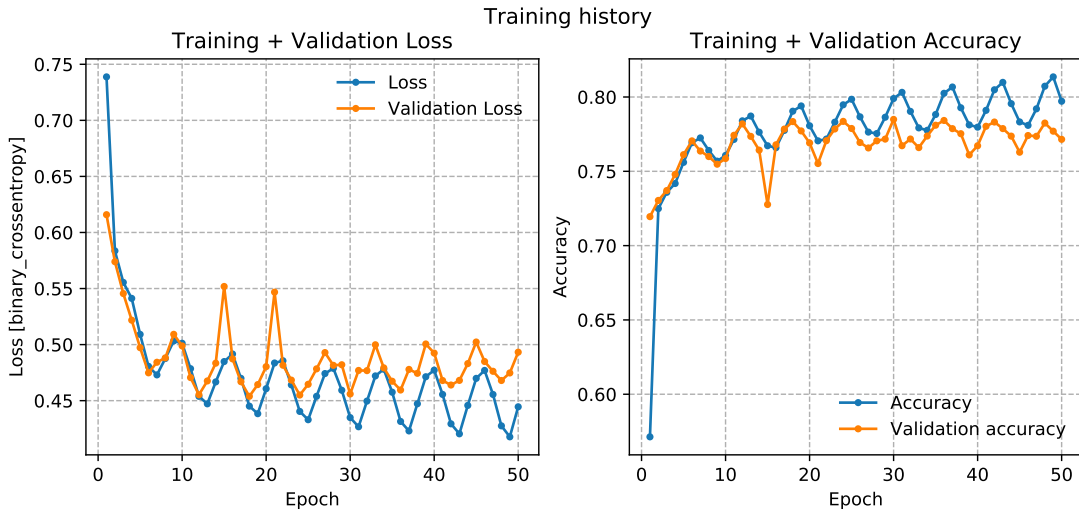
Figure 4.1: Training history of the low-cut VGG13. The wavy behaviour is an effect of the CLR policy.
