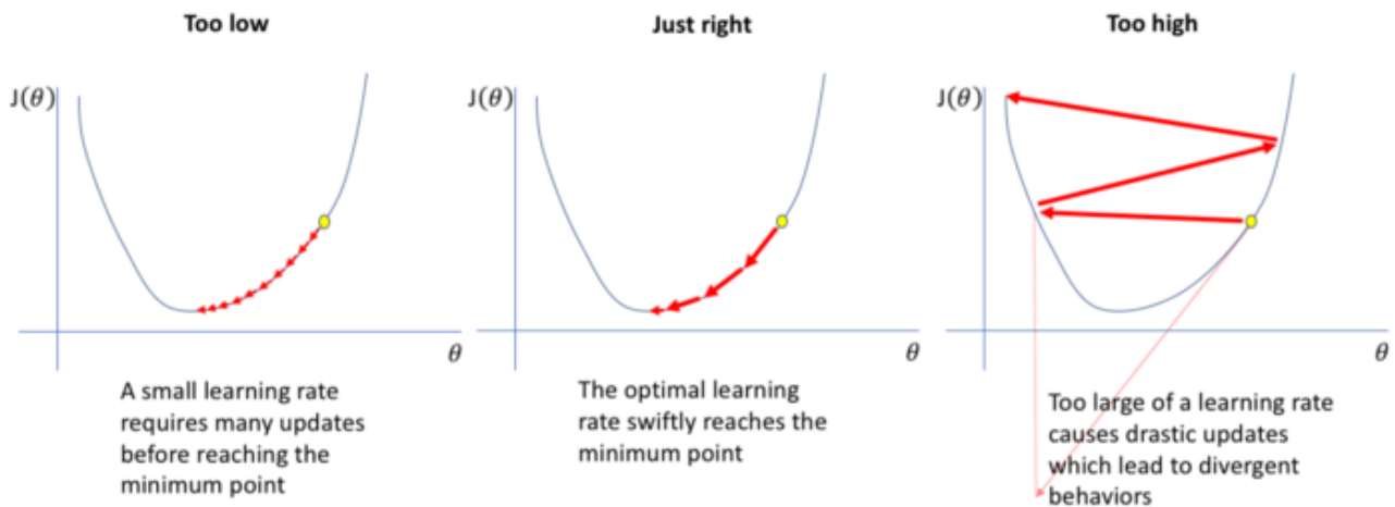
Figure 3.2: 1-D representation of the impact of different values of LR on the minimization of a loss function J(\theta) . Image courtesy of J. Jordan.
